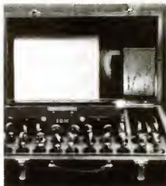
The mysterious so-called IBM portable contained 20 vacuum tubes.
